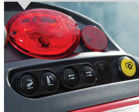
Fender mounted PTO, hydraulic spool valve and linkage controls.
