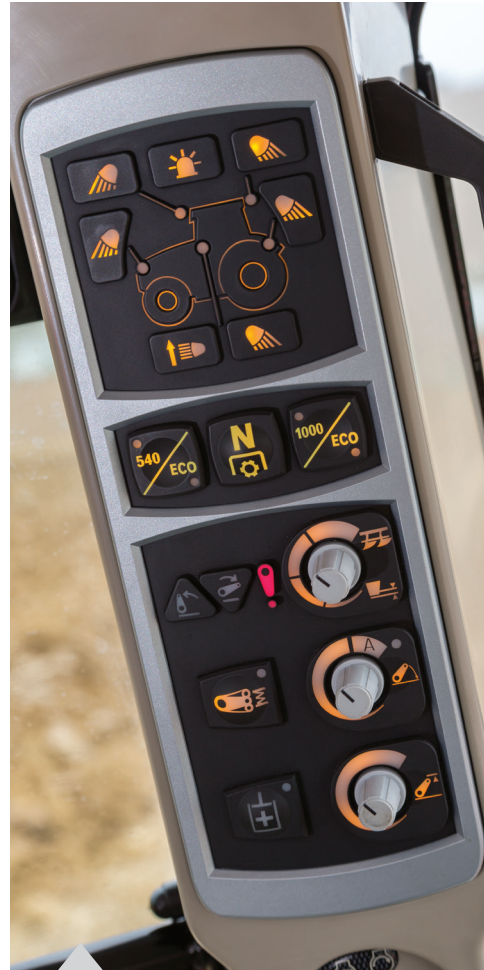
Pillar mounted PTO speed selection controls and linkage controls.
