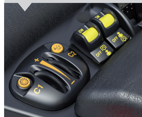
Fender mounted PTO, hydraulic spool valve and linkage controls.
